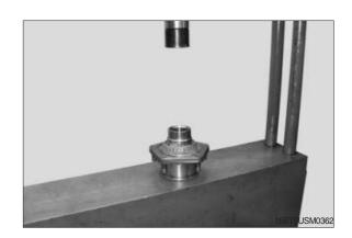
(16) Fit the housing perpendicularly onto the wheel shaft.
