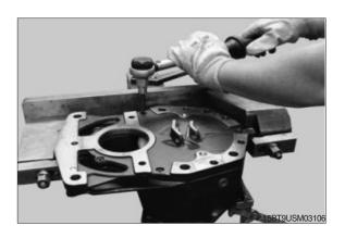
(23) Manually check the wheel shaft for smooth running.It shall be possible to move the wheel shaft easily by hand.
