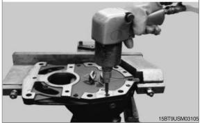
(22) Tighten the 8 Allen bolts to a tightening torque of 9.5 Nm.
