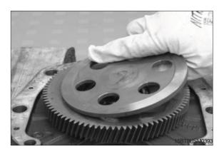
(10) Fit the inner disc carrier onto the spur gear ) by hand.
