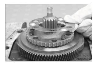
(13) Insert the 6 Torx bolts into the fixing plate and screw them down into the spur gear tighten them by hand.
