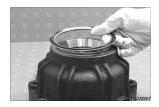
(2) Drive up the sealing ring into the transmission housing against the block.
