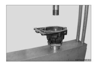
(17) Place the taper roller bearing onto the seat of the wheel shaft.
