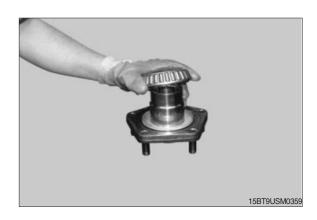
(13) Press taper roller bearing on gear wheel side onto gear shaft using lever press and tool.
