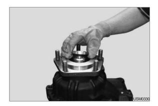
(5) Place the housing on the press table with the mating surface facing downwards.
