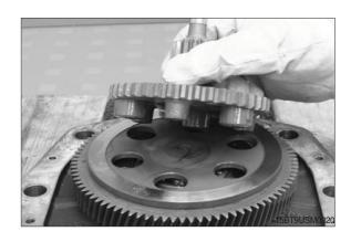
(9) Manually remove the pressure disc from spur gear.
