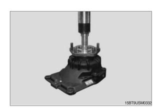
(7) Remove the planet carrier from the housing.
