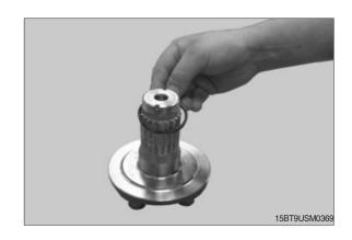
(22) Coat the toothing of the planet carrier and the o-ring with Klüberplex BEM 34-132 (Klüber Lubrication) or Optimol White Paste T.
