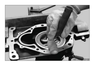
(19) Fit the housing cover to the housing by hand.
