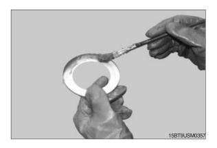
(11) Slide the Nilos ring onto the wheel shaft.
