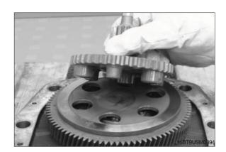
(11) Insert the 3 pressure springs 1.6 x 8.0 x 21.5 into the inner disc carrier by hand.
