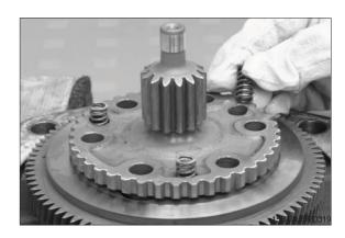
(8) Manually remove the inner disc carrier from the pressure disc.
