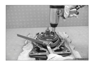
(6) Manually remove the retaining plate from the spur gear together with the 6 Torx bolts.
