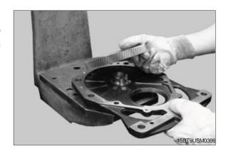
(3) Press the spur gear onto the housing cover.
