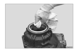
(6) Drive the wheel shaft side bearing cup of the taper roller bearing into the bearing seat.
