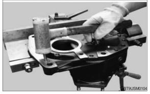
(21) Screw the 8 Allen bolts into the housing cover by hand and slightly tighten with a compressed air screwdriver.
