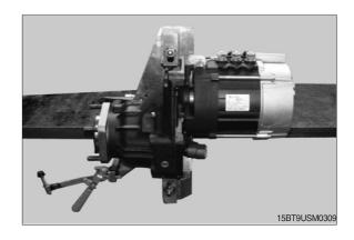
(2) Fasten the motor to suitable lifting gear using approved attachment equipment.
