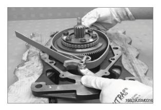
(5) Hold the spur gear tight using the strap wrench. Undo the 6 Torx bolts.
