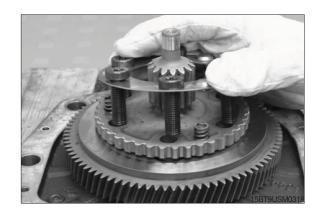
(7) Manually remove the 3 pressure springs 1.6x8.0x21.5 from the spur gear.
