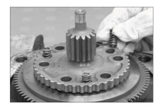
(12) Place the fixing plate over the pressure spring by hand. The springs shall be firmly seated in the recesses in the retaining ring.
