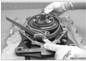
(14) Hold the spur gear tight using the strap wrench. Tighten the 6 Torx bolts to a tightening torque of 70Nm using an adjustable compressed-air screwdriver.
