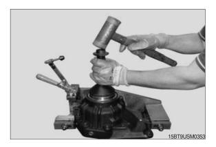
(7) Coat the inner lip of the shaft sealing ring with multipurpose
