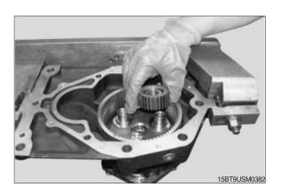
(35) Drive in the planet gear including the cylindrical roller bearing until reaching the limit stop. Use a hammer and a striking mandrel. Drive in the remaining two preassembled planet gears by using the same method. Note the correct meshing of the teeth of both planet gears and ring gear.
